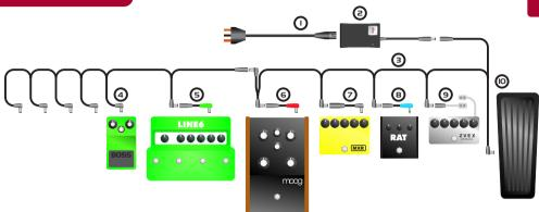
O Connect the AC Mains cable to the Powerstation ③ You can use the Powerstation anywhere in the world. The cable is a standard C7 (also known as figure 8) detachable type.
